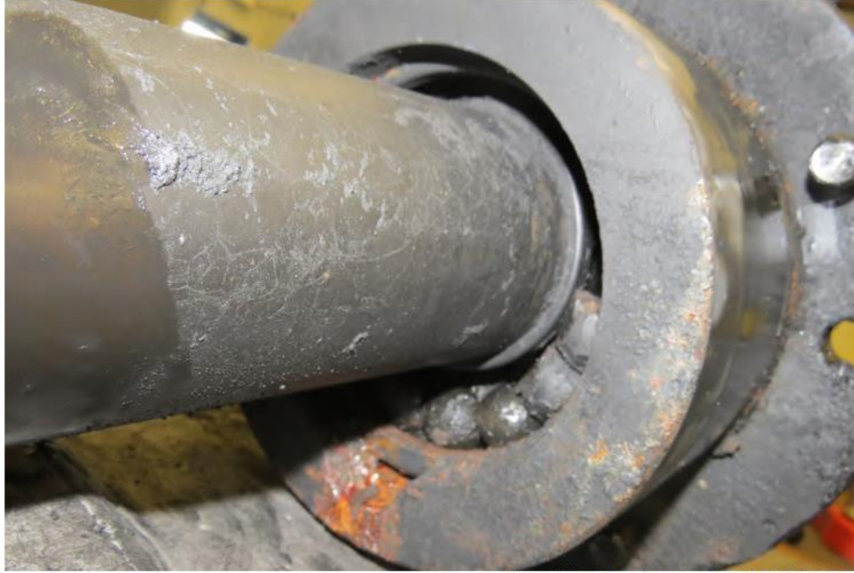
Fig. 5 – Bearing Housing with Loose Ball Bearings
