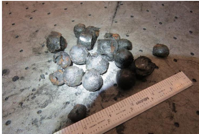
Fig. 8 – Outboard Bearing Balls
