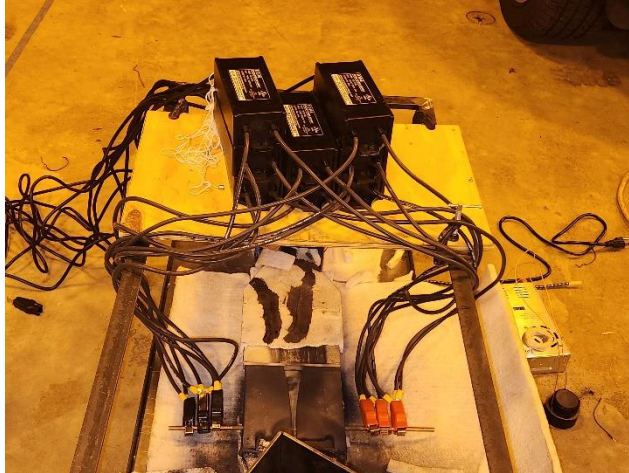
Fig. 26 - Power Delivery System
