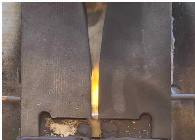
Fig. 18 - 2400W Gliding Arc with CO 2 and Iron Oxide Combustion Test
