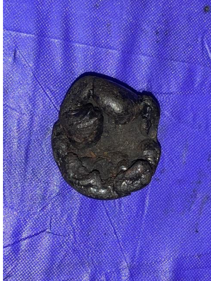
Fig. 9 – Bearing Ball with Void
